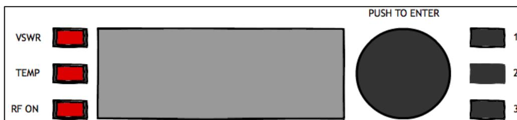
The buttons on the right of the scroll knob interact with the menu system, usually button 1 is 'exit', button 2 is 'help' and button 3 is 'meters'. In some menus however their functions change. The indicators on the left show RF on, and VSWR and TEMPerature warnings.
